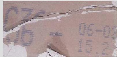
Marking: KNAUF – WuHu, China – ASTM C36 – [DATE] [TIME]
