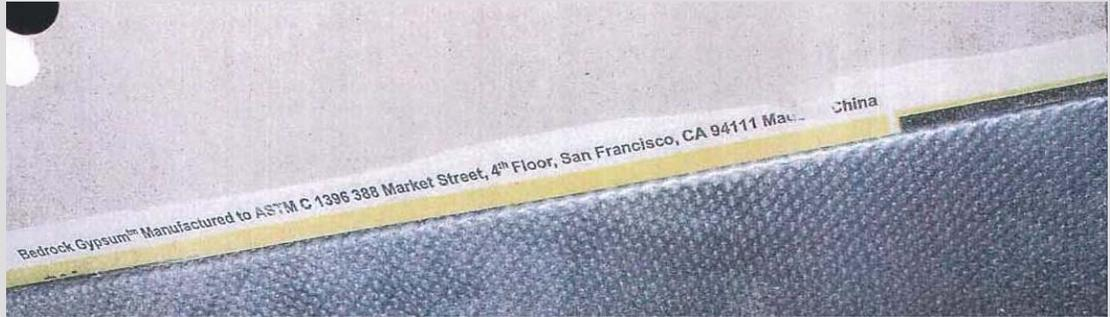
Marking: Bedrock Gypsum™ Manufactured to ASTM C 1396 388 Market Street 4<sup>th</sup>
