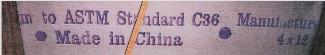
Marking: **Manufactured to Conform to ASTM Standard C36**
