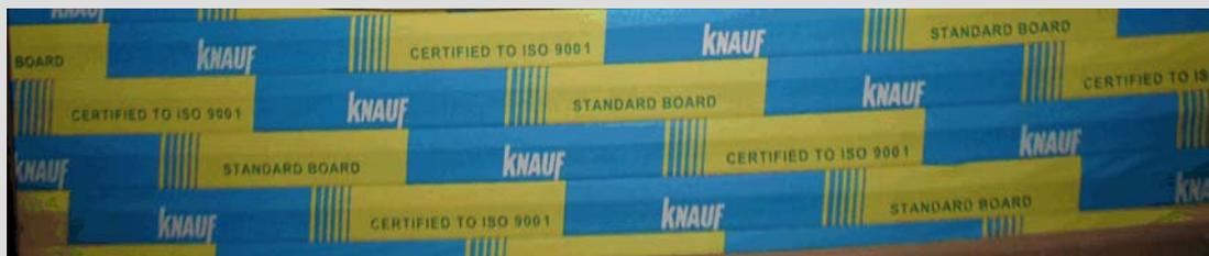
Marking: “ KNAUF CERTIFIED TO ISO 9001 KNAUF STANDARD BOARD “
