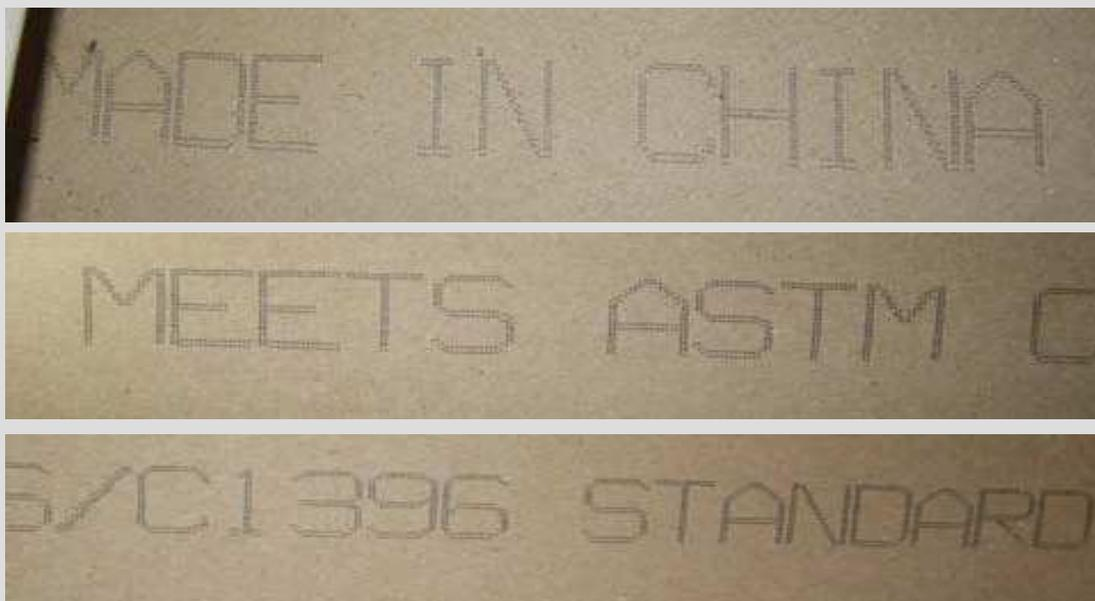
Marking: **MADE IN CHINA MEETS ASTM C36/C1396 STANDARD**
