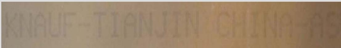
Marking: **KNAUF – TIANJIN CHINA – ASTM C36**
